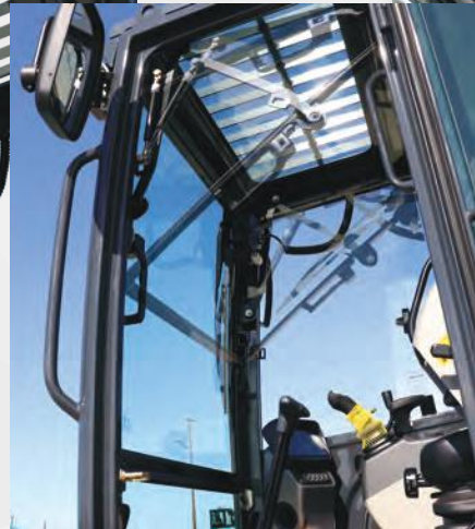
Enclosed cab with A/C, Touchscreen Monitor, Rock Guard and removable windows
